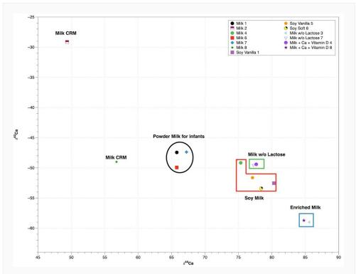
Figure 4: Isotopic composition of Ca in 13 milk samples measured. Ca isotope ratios are presented on a  $\delta$ -scale ( $\delta^{44}$ Ca vs.  $\delta^{42}$ Ca). More negative  $\delta$ -values correspond to a lower  ${}^{43}$ Ca/ ${}^{44}$ Ca isotope ratio, i.e., an enrichment of the heavier Ca isotopes, compared to the reference material of Ca stock standard.
