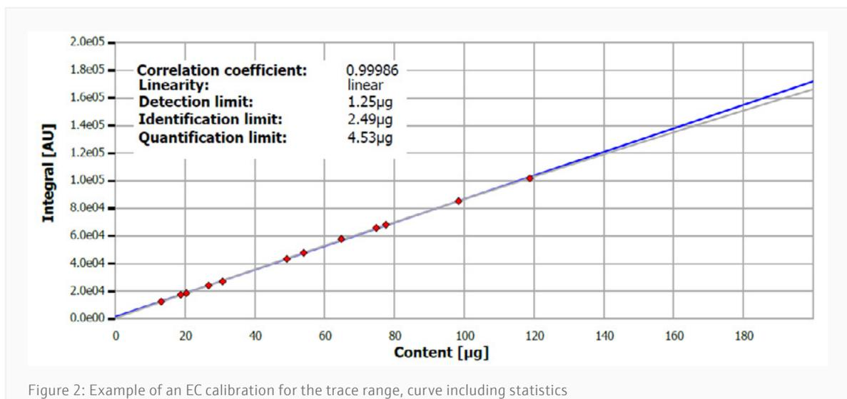
Figure 2: Example of an EC calibration for the trace range, curve including statistics
