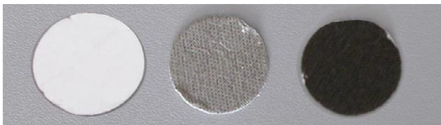
Figure 1: Filter samples, uncontaminated (a.) blank filter, (b.) slight contamination, (c) heavily contaminated filter
