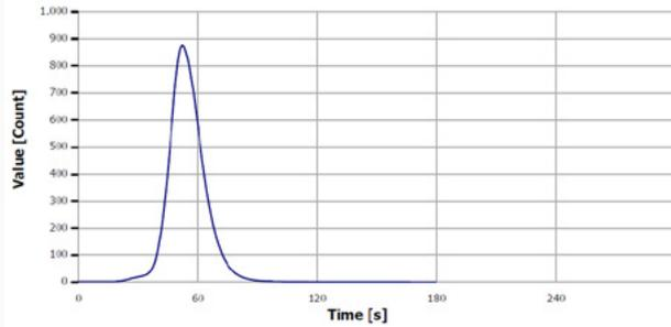
Figure 8: EC analysis curve of "EC standard 1.01 g/kg"
